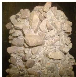
15% Sulphuric acid attack on high-strength concrete after 20 weeks
